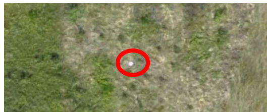
Figure 18 – Example of identification of a QCP (plastic plate) on the point cloud
